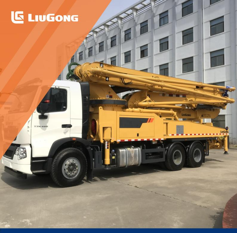
Chassis Brand Emission Regulation Max. Concrete Output (L/H) Max. Concrete Pressure (L/H) Max. Vertical Reach Concrete Slump SINOTRUK Optional 120/80 m<sup>3</sup>/h 7/11 MPa 37.75 m 120-230 mm
